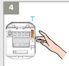
**TOGGLE MODE (**T): Recommended for switch applications. The first detection activates the relay output and the second detection deactivates it. In door applications the door remains open after the first activation.
